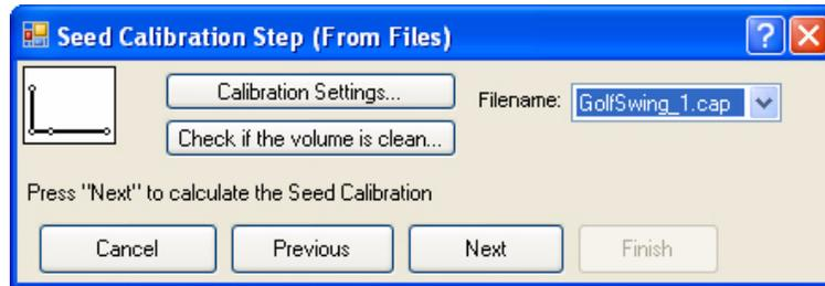
The L-Frame defines the capture volume's coordinate system. All cameras do not need to see the L-Frame to obtain a successful calibration.
