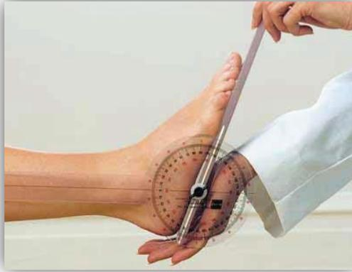
This handheld, transparent goniometer standardizes the clinical assessment of ankle dorsiflexion. Structure allows examiner to control entire forefoot, subtalar joint and ankle joint, preventing unacceptable pronation during measurement. The plantar platform acts as a goniometric mobile arm, helping to minimize the variables in technique common with single-plane goniometers. Goniometer has a durable polycarbonate base.
