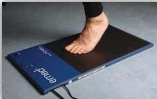
Emed Pedography Platforms are accurate electronic systems for recording and evaluating pressure distribution under the foot in static and dynamic conditions. The Emed systems belong to the family of novel pedography measurement platforms. All scientific Emed platforms operate with calibrated capacitive sensors.
