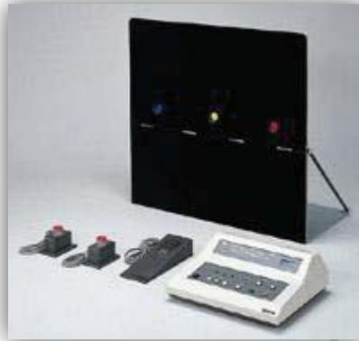
This device measures person's reaction time to the sound and color or the combination of both, as a stimulus. After receiving the visual stimulus the reaction time is measured and the results are used to study the effects of drugs, fatigue, lack of sleep, nutrients, etc. on physiological functions. Calculating method of assessment criteria and its interpretation is available in the user manual.
