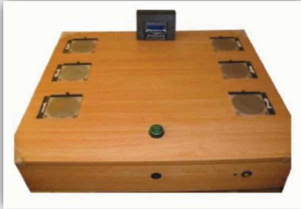
This system includes hardware for the implementation of various movement patterns, and software to collect and analyze data. The aim of this device is to study research variables in the field of motor learning including time of movement, reaction time, the role of feedback, observational learning, etc.
