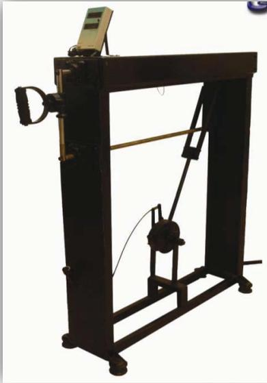
This machine as a resistance device can improve both muscle strength and Zuki skill. Using a lever, the angular momentum caused by resistance section is attached to a rod in a sinusoidal path. Sinusoidal movement of the device may cause high punching resistance at the beginning, low resistance at the middle and an increase at the end of the movement. this pattern causes a ballistic movement.
