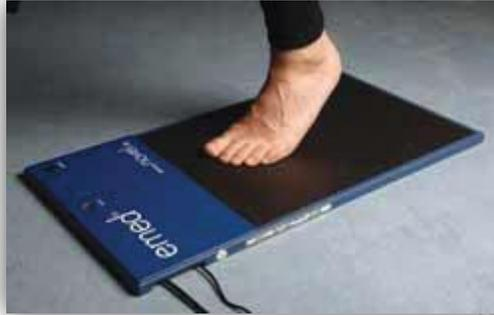
Emed Pedography Platforms are accurate electronic systems for recording and evaluating pressure distribution under the foot in static and dynamic conditions. The Emed<sup>®</sup> systems belong to the family of novel pedography measurement platforms. All scientific Emed<sup>®</sup> platforms operate with calibrated capacitive sensors.
